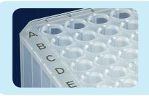
All plates have easy-to-read, laser-marked alphanumerics with an A1 orienting corner. Deep well plates have raised rims for better sealing and less chance of cross-contamination between wells.
