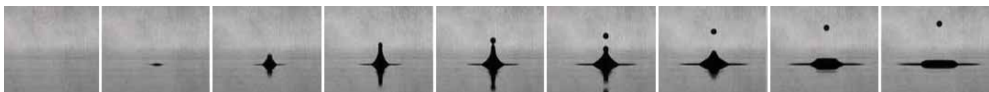
FIGURE 1: Precise amount of acoustic energy is supplied to the fluid creating a single drop
