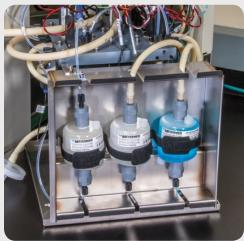
The ZE5 comes with two sets of sheath and waste tanks that are hot-swappable anytime one set is used up. The tanks are driven by a low vibration, high-pressure fluidics module that provides uninterrupted operation throughout the day.
