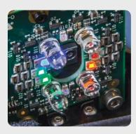
A series of LEDs of different wavelengths illuminate the light path. The amount of light reaching each PMT from the different wavelength LEDs is determined by the filters that are in place. The detected PMT signal is compared to a reference to determine whether the expected filter set is in place. If the signals do not match, a warning will be displayed at the relevant PMT(s).
