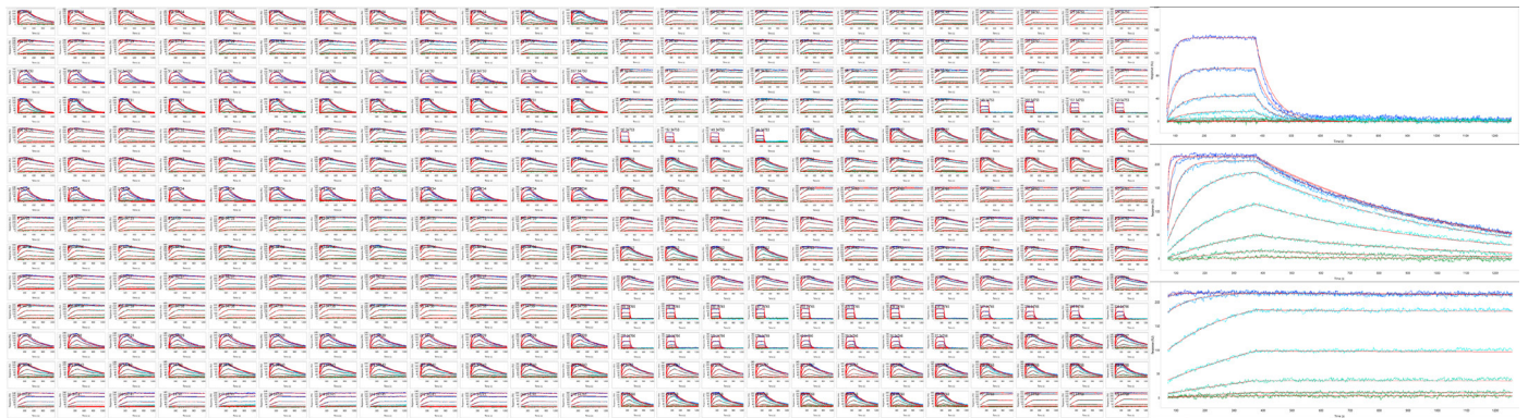
Simultaneous kinetic analysis of 384 antigen/antibody binding interactions using Array SPR (Left), with (Right) Enlarged view of the data from three spots showing antibodies that bound their target with diverse kinetics (low, medium, and high affinities, from top to bottom).
