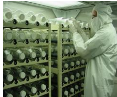
Surface Coated Large Scale Cell Production Vessels
