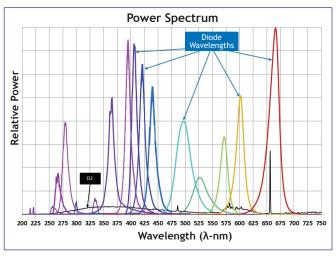
Conventional bulbs provide a broad spectrum of low-intensity energy, much of which is not useful. Users have dealt with sub-optimal solutions that require frequent replacements, hazardous waste handling, and potentially dangerous wavelengths. LEDs offer orders-of-magnitude higher power output within specific targeted wavelengths for disinfection, analysis, spectroscopy and fluorescent imaging.
