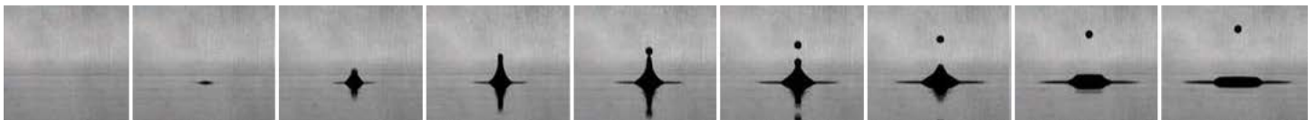
FIGURE 1: Precise amount of acoustic energy is supplied to the fluid creating a single drop.
