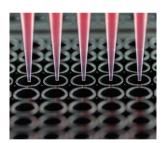
**1.** Dispense the Sample Solution and Diluent into a Verification Plate and mix.
