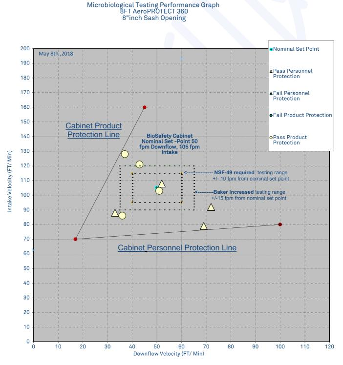
**RESULTS:** AeroPROTECT 360° has passed all Product Protection and Personnel Protection tests conducted within and beyond both the NSF International Standard 49 requirements as well as the Baker Safety Range.
