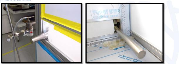
6. Staggered the panes leaving smaller openings at 4 locations. Tested the middle 2½" opening for product protection.
