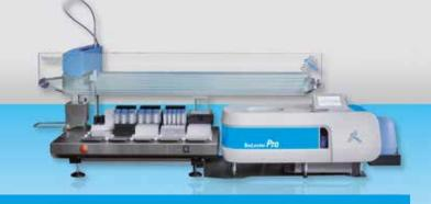
The combination of a micro bioreactor with a liquid handling robot, RoboLector®,
