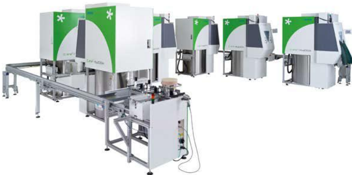
Connection of several ASKION C-line® hermetic storages to one fully automated biobank by using the external automation (rail system with shuttle and transfer station)
