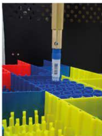
Pick-and-Place robot with one single sample above a tray at cryogenic temperatures (left), gripper changing system of HS200 M/L (middle) and SBS rack gripper (right)
