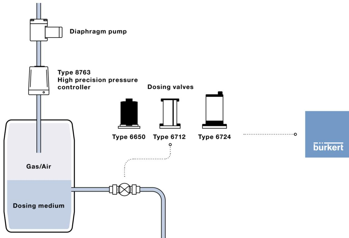
We coordinate the valve and pump as well as the length and diameter of the supply lines, thereby ensuring the valve always switches exactly and in a consistent manner – even after routine replacement of the valve.
