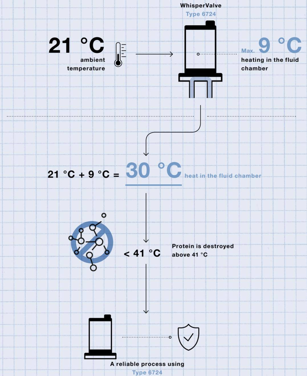
**Result:** When the medium is stationary, the maximum heat input into the medium is 9 °C. As a result, the temperature in the fluid chamber rises to 30°C and remains safely below 41 °C. During normal operation, there is flow when the valve is switched on, which causes virtually no heating of the medium.
