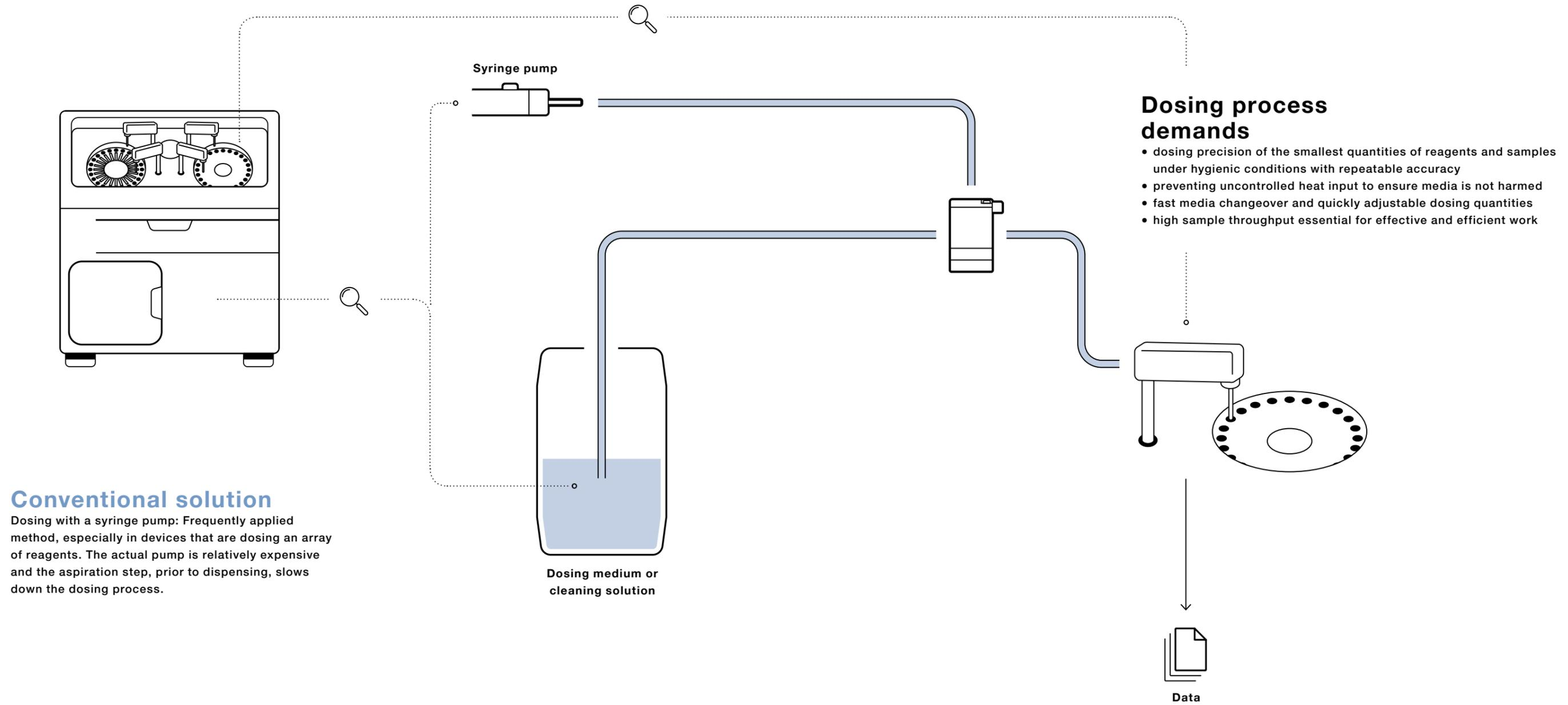
**/ Fast, precise and consistent dosing / Bürkert's time-pressure dosing technology helps to speed up the dosing process and increase the efficiency of your analytical device. In addition, the design of the valve prevents uncontrolled heat input into the medium and helps you achieve accurate test results. Good to know: We adapt Bürkert system solutions to your requirements – or develop an individual solution together with you.**
