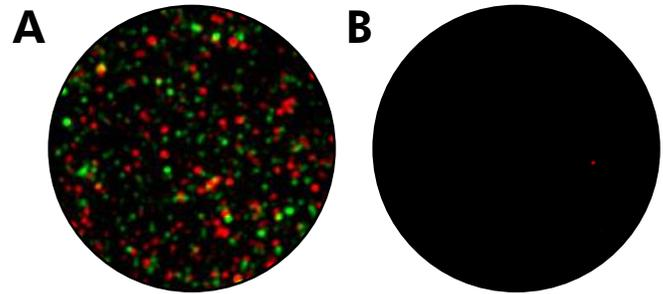
**Figure 4: The ExoView Isotype Control is a built-in check of each assay.** EVs are incubated on a chip with anti-CD81 capture antibody and stained with fluorescent anti-CD81 (green), anti-CD63 (red), and anti-CD9 (blue) antibodies. (A) CD81 capture spot showing bound vesicles counterstained with fluorescent antibodies and (B) Isotype Control from same chip showing very limited non-specific response.
