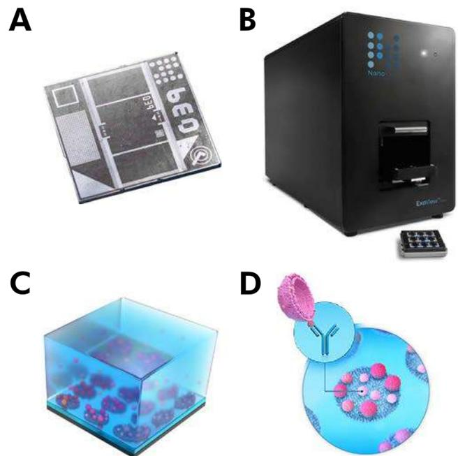
**Figure 3: The ExoView microarray chip works through EV affinity.** (A) Photograph of the microarray chip with specific affinity antibody spots. (B) Photograph of the ExoView instrument, in which the microarray chips are read out. (C) Sample incubated on ExoView microarray chip. (D) EVs that carry corresponding antigens bind to the antibodies on the microarray chip and are ready for analysis.
