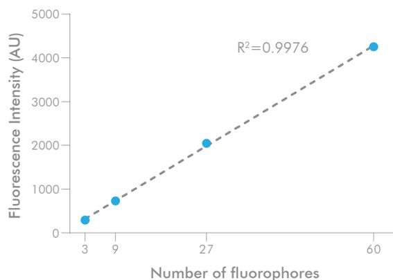
**Figure 2: Fluorescence signal measured by ExoView is linearly proportional to the number of fluorophores.** Gattaquant DNA origami nanostructures with 3, 9, 27, or 60 fluorophores were measured by ExoView.
