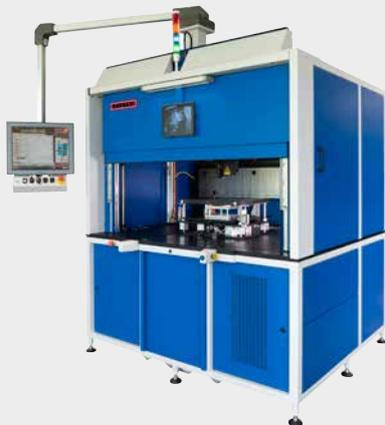
MAXI is a modular, universally applicable laser welding system and specializes in large components. It can be equipped in many different ways as a manual workstation and can be adapted to customer-specific applications and processes.
