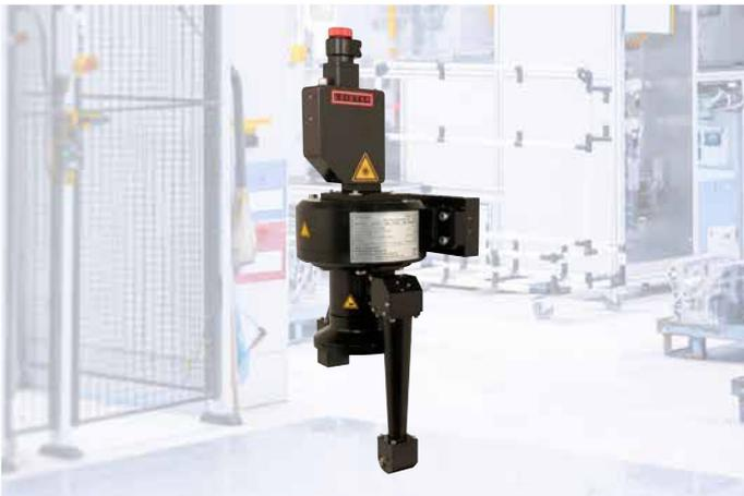
The Rotation Optic is used for sequential welding of rotationally symmetric components. It is operated exclusively with a fiber laser, which can be adjusted in different diameters via an M-shape DOE. A synchronous electric motor with hollow shaft and incremental position measuring system is integrated into the optics and moves a cantilever arm (rotor) around the component. The laser beam is deflected towards the center by an adjustable mirror at the end of the rotor.
