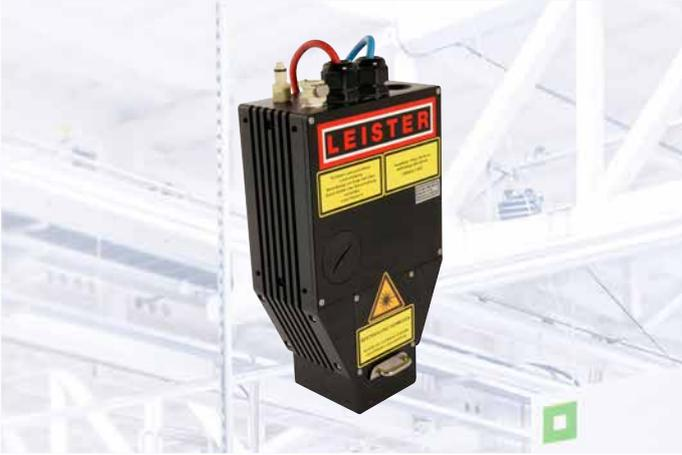
The LineBeam is the ideal beam source for mask welding. It generates a line with almost constant power density distribution, resulting in a consistent welding pattern. The LineBeam is a compact system consisting of a diode laser and directly coupled optics. The optical components of the system can be adjusted to different line lengths.
