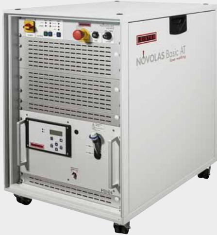
The NOVOLAS™ BASIC AT welding system is designed for integration into complex production lines. Due to its consistently modular design, it can be configured very well for different requirements.
