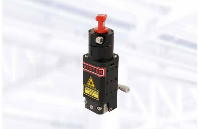
The Roller Optic requires no additional clamping technology. With the Roller Optic a linear laser beam is guided through a glass roller, which is both the pressure tool and the last optical element. The roller, which is supported on two sides, can produce weld seam widths of about 3.0 – 6.7 mm. Due to the pendulum bearing of the roller, small irregularities in the axial direction can be compensated.
