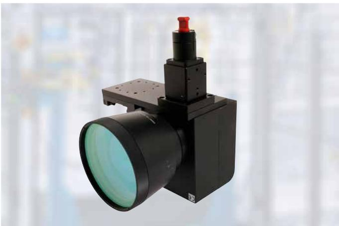
The Scanner Optic is characterized by the integrated option of movement and is mainly used for quasi-simultaneous welding. Two movable mirrors guide a spot laser beam along a programmed contour. The size of the working field can be adjusted by different focusing lenses. Like all optical components, the Scanner Optic can be installed in all Novolas™ laser welding systems.
