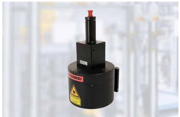
With the Radial Optic, rotationless laser welding is possible without additional clamping technology. Radial welding is suitable for rotationally symmetrical components that are difficult to rotate themselves. The laser radiation is deflected onto the circumference of the components by a conical mirror. This allows components with a diameter up to 68 mm to be welded simultaneously, which results in short cycle times and high throughput.
