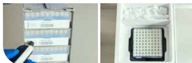
CryoBox being read with a CryoBox Tracker
