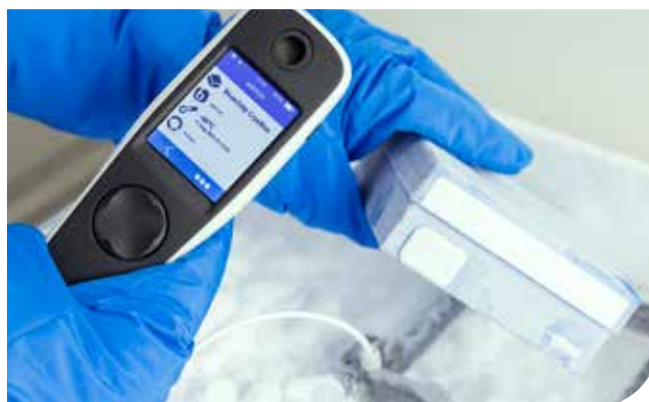
Universal CryoBox being read with a CryoBox Tracker
