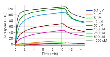
Overlay plot displays a full kinetic characterization using COOH Agile biosensors. A concentration series of small molecule SPD304 is measured against immobilized TNF $\alpha$ , a cell signaling protein used as a therapeutic target. These curves show the concentration dependence of the biomolecular interaction, and the evaluation software provides  $k_{on}$ ,  $k_{off}$ , and  $K_{D.}$
