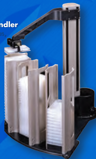
ProNEDx™ Ultimate-Performance Robot (450mm radial X 250, 500, or 750mm vertical strokes)
