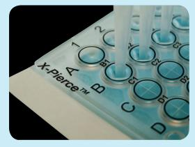
Scored for easy piercing. Repositions to protect well contents when probe is removed.
