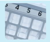
2 ml and 384-well plates have square wells with rounded corners that enhance sample recovery and minimize cross-contamination by reducing capillary wicking.
