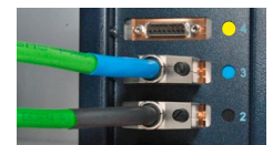
Multi TEC Control (MTC) with three inserted slot modules and two connected devices with corresponding color
