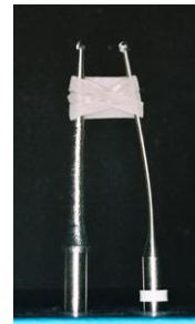
Figure 2. Stiff shaft of Munce Discovery Bur compared to flexible shaft of the smallest Mueller bur (~ #2 round).
