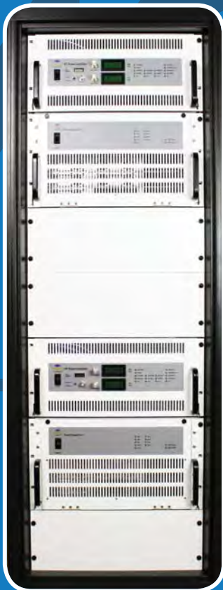
72.75MHz, 2 x 4kW amplifiers and power supplies
