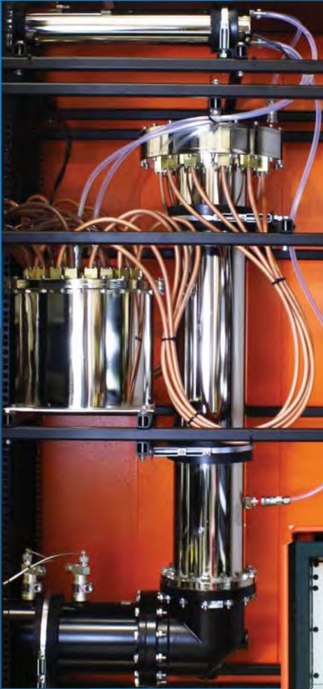
340kW final combiner
